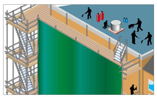
**Figure 12** In this job, hot work on the roof and window renovation using blowlamps and substantial amounts of flammable materials mean the fire risk is high. Escape via ladders inside the sheeting could be difficult so unsheeted external access is provided at one end. Some scaffold components have been omitted for clarity (such as roof edge protection). The escape route must lead away from the enclosure where practicable
