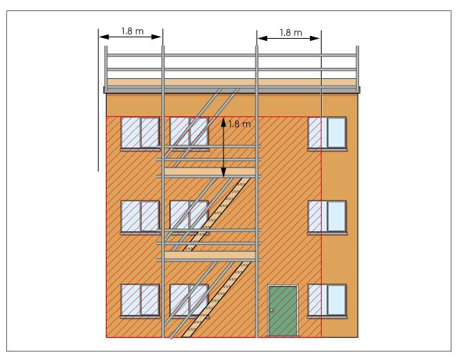
**Figure 11** Temporary scaffold-based escape routes need to be protected from fire inside the building. The windows inside the shaded area need to be blocked off with fire-resisting material and the ground- and first-floor doors need be fire-resistant and self-closing
