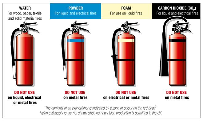
**Figure 17** A selection of fire extinguishers. Fire extinguishers complying with BS EN 3 are red with a coloured zone identifying the extinguishing agent. For example, blue signifies a dry powder fire extinguisher. The contents of an extinguisher are indicated by a zone of colour on the red body.
